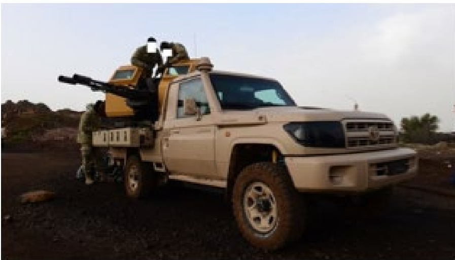
Turkish troops' new 'hybrid vehicle' spotted in Afrin. The 4X4 platform is equipped with ROKETSAN – manufactured ballistic armor protection and ZSU-23-2 23mm autocannon. 49
