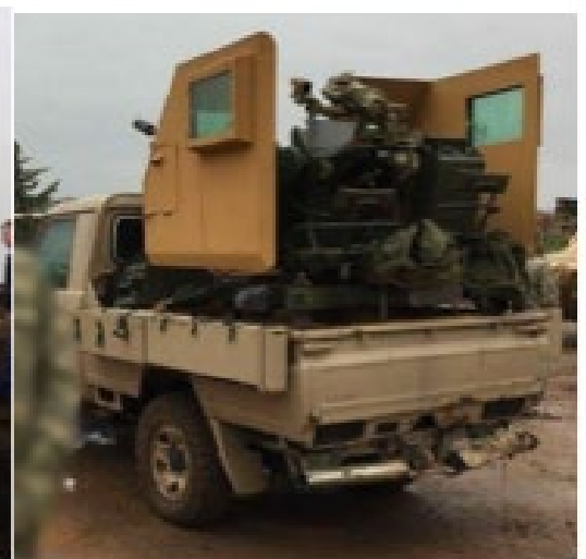
Turkish troops' new 'hybrid vehicle' spotted in Afrin. The 4X4 platform is equipped with ROKETSAN – manufactured ballistic armor protection and ZSU-23-2 23mm autocannon. 49
